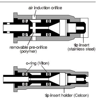
pressure or vacuum created within the nozzle will draw air into the spray solution, forming air bubbles. The air and liquid exit the nozzle as a larger spray droplet with the potential to get more pesticide product to the target and reduce drift.
