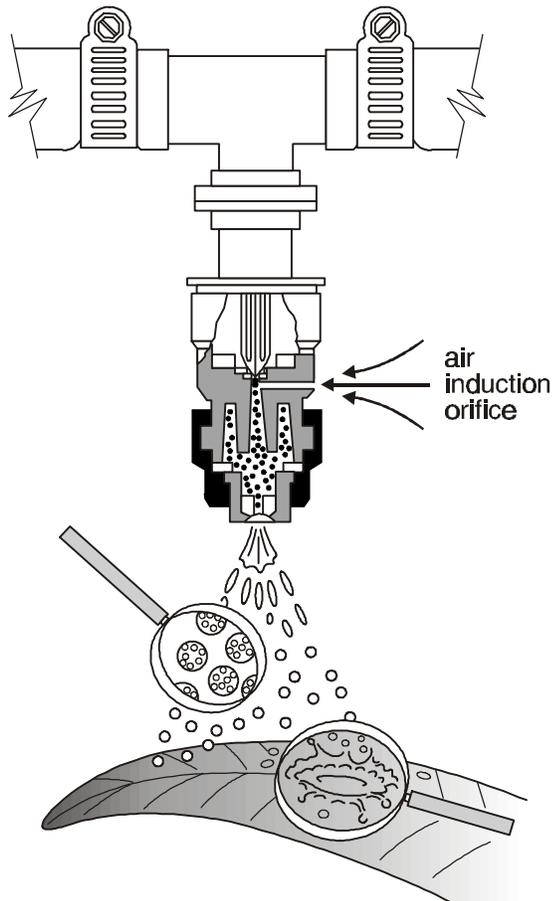
pressure or vacuum created within the nozzle will draw air into the spray solution, forming air bubbles. The air and liquid exit the nozzle as a larger spray droplet with the potential to get more pesticide product to the target and reduce drift.
