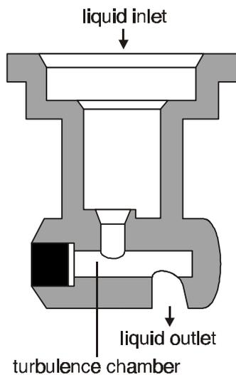
**Figure 5. Turbo Flood Nozzle.**
